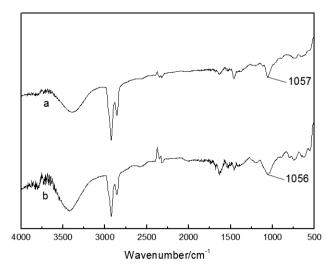
Fig. 11. Infrared spectrum of DDPB(a) and the extracted species(b)
