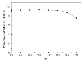
Fig. 6. Effect of pH on the extraction of Pd(II)
