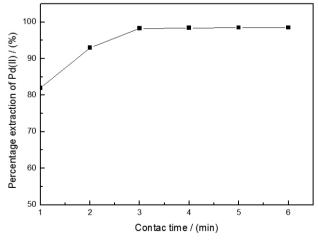
Fig. 3. Effect of contact time on extraction of Pd(II)
