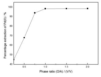
Fig. 4. Effect of phase ratio (O/A) on extraction of Pd(II)
