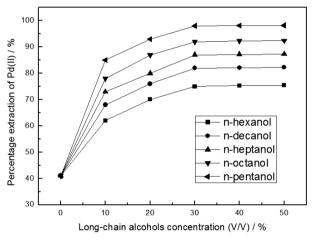
Fig. 1. Effect of different long-chain alcohols on the extraction percentage
