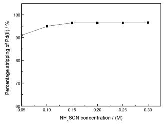
Fig. 7. Effect of stripping reagent concentration on the stripping of Pd(II)
