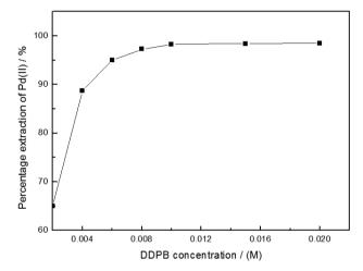
Fig. 2. Effect of extractant concentration on the extraction of Pd(II)
