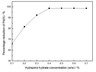
Fig. 8. Effect of hydrazine hydrate concentration on the reduction of Pd(II)
