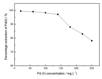
Fig. 5. Effect of initial palladium concentration on extraction of Pd(II)
