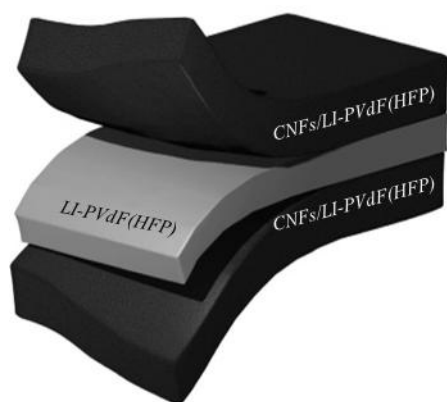
Figure 2: Schematic representation of the sandwich configuration of the CNFs actuator, composed of two electrode layers and one electrolyte layer.
