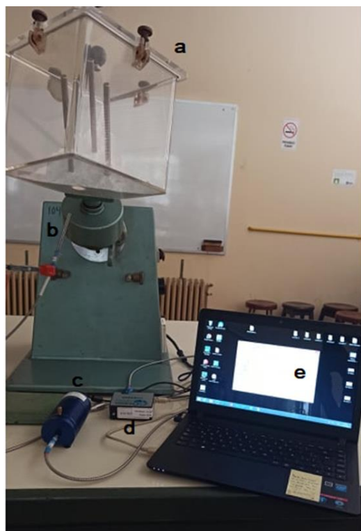
a: blender machine; b: Probe; c: Source; d: Detector; e: Laptop
